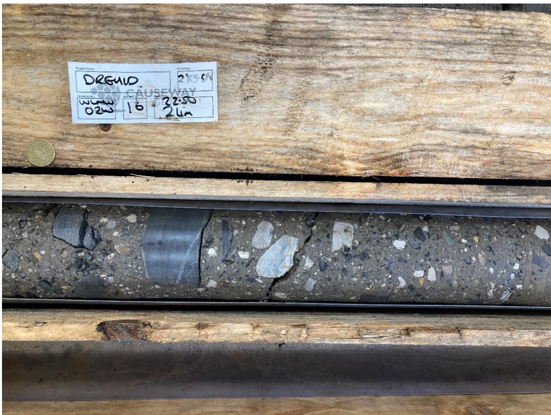
Photo 4 Glacial Till Core, Borehole MW02B (Peg ID: WLMW02W), 22.5-24.0 m Depth
