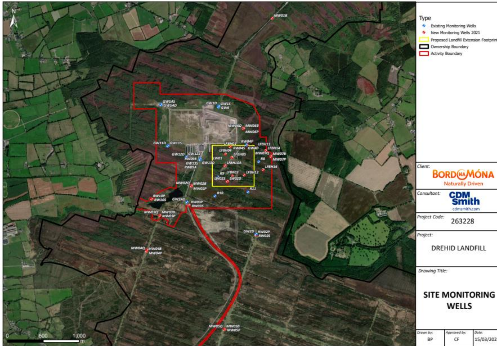
Figure 7-2 Locations of Piezometers/Monitoring Wells Installed for the Updated SI (2020-2021)
